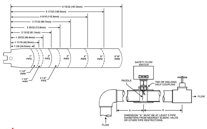
**CAUTION:** The paddle must be trimmed at the dotted arc. It must not touch the pipe or any restrictions when installed.
